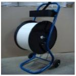
Carriage of polypropylene fastening tape. It facilitates transporting of PP tape on-site.
